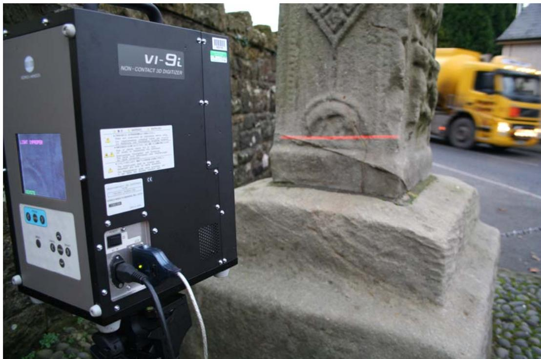
**Figure 2. A.** Small scale laser scanner – Konica Minolta Vi9i, Donaghmore Cross, Northern Ireland
