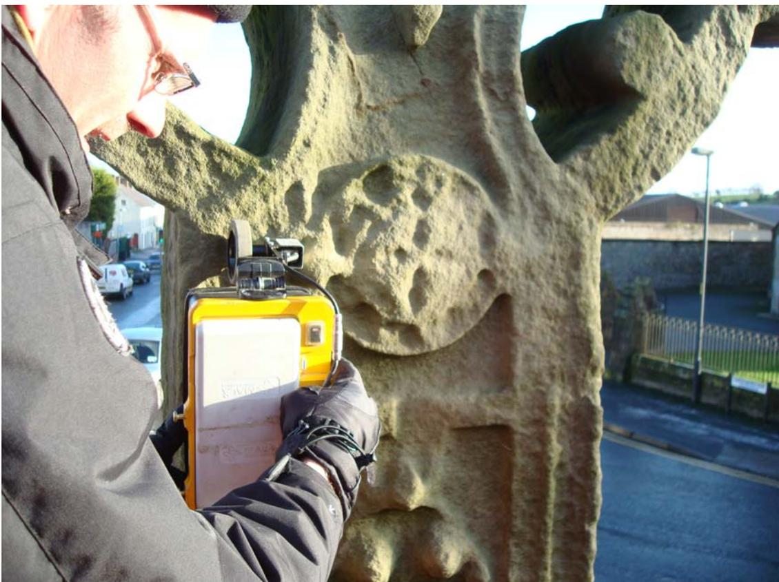
**Figure 7.** Photograph of High Resolution Ground Penetrating Radar being used on site, Donaghmore Cross, N.Ireland.
