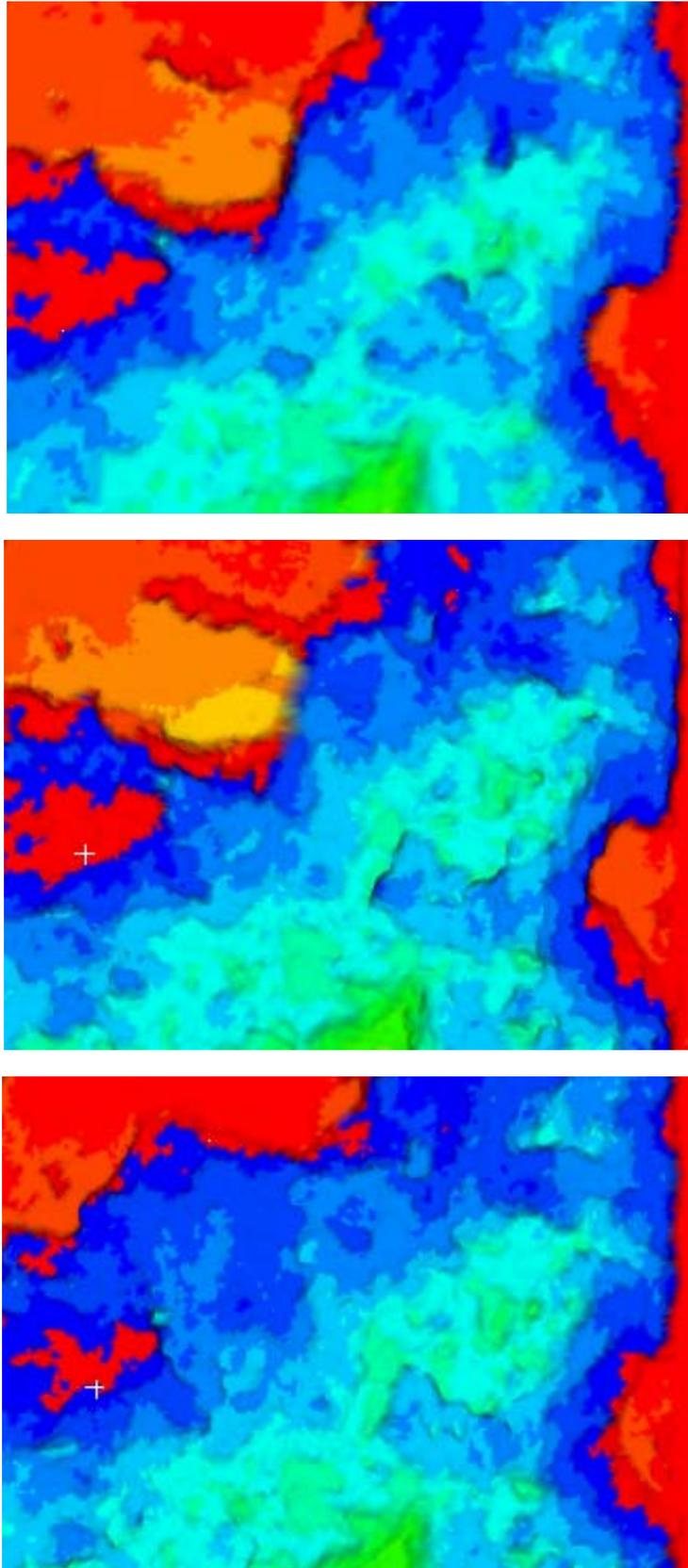
**Figure 5.** Successive DEMs, **A. 2006 B. 2007 C. 2008** of a small 10cm x 8cm area of Worcester College facade, Oxford, showing surface swelling, yellow (B) and material loss (C). (Yellow high, green low).
