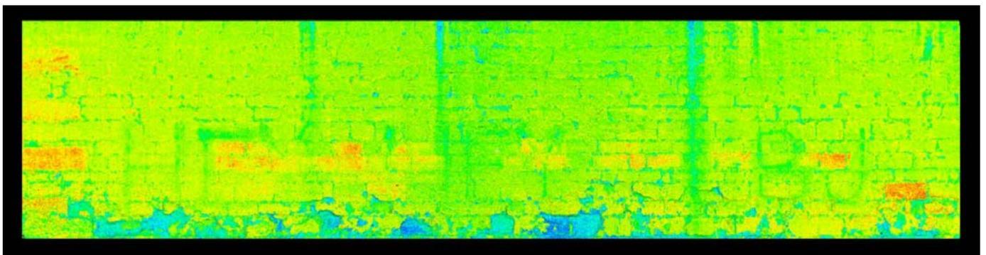
**Figure 3 A.** LiDAR scan of a 13.6m x 3.2m section of limestone wall, New College, Oxford. This image is made up of 100,000s of individual points artificially coloured based on their reflectance value. Blue – High Reflectance, Red – Low reflectance.
