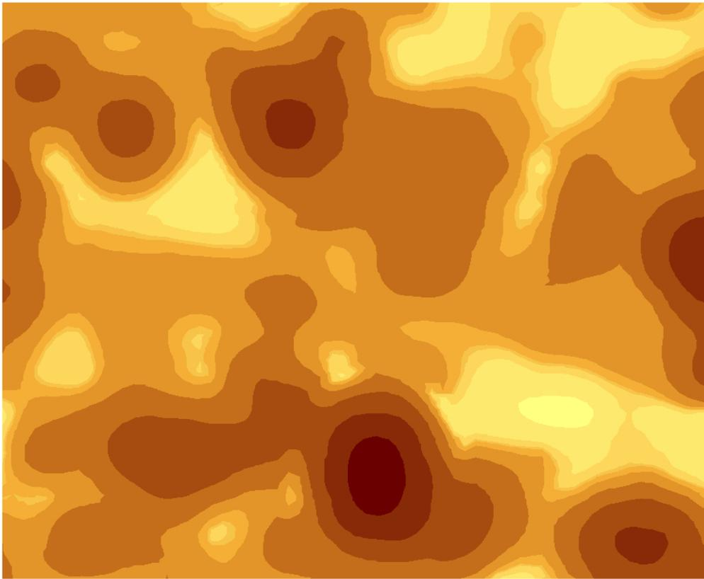
**Figure 6.** Permeability map created using GIS software, of a limestone ashlar block (40cm x 35cm).
