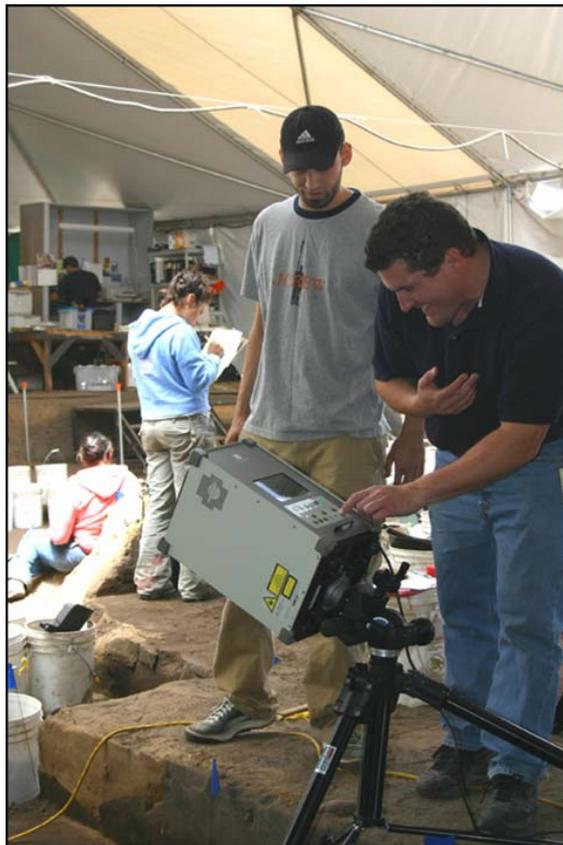
Figure 3. Photograph of archaeologists using a 3-D scanner at a prehistoric archaeological site in California (courtesy of Statistical Research, Inc.).
