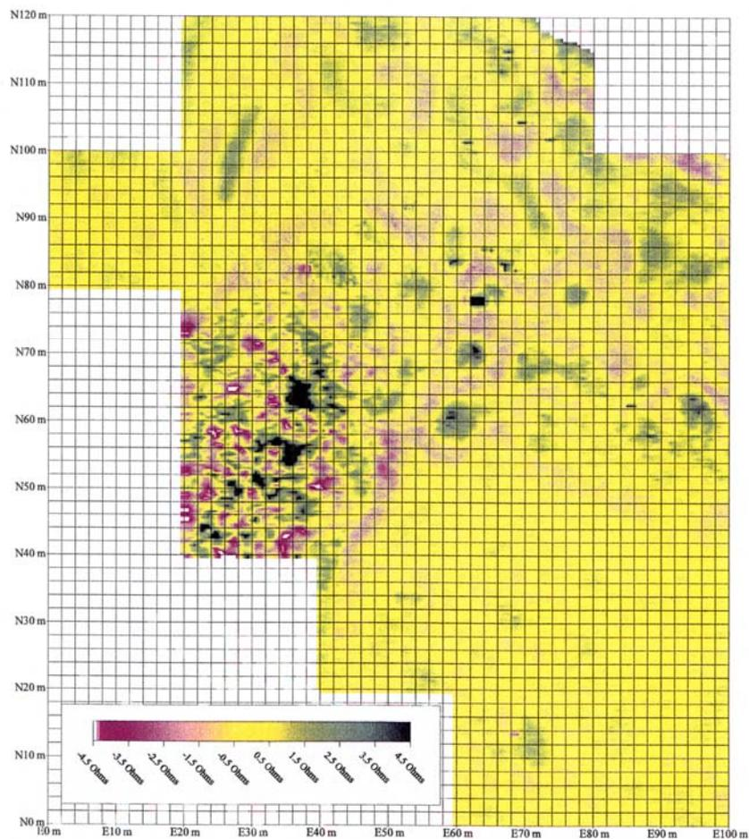
Figure 2. An electrical resistivity map of a prehistoric shell midden site prepared using Surfer, version 6.01. Areas depicted in black, red and white depict potential buried cultural features (from Grenda et. al. 1998).
